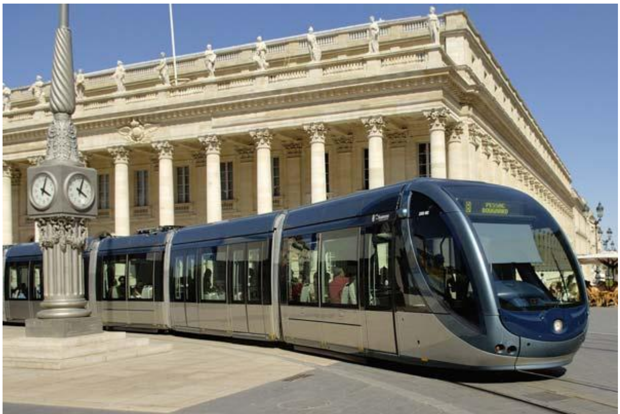
Bordeaux tram operating using the APS system through the city centre
